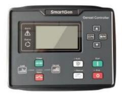
SmartGen HGM series controller, integrating digital, intelligent and network techniques, is used for automatic control and monitoring system of genset. It can carry out functions of automatic start/stop, data measurement, alarm protection and three "remote" (remote control, remote measure and remote communication). The controller uses LCD display, optional display interface including Chinese, English, Spanish, Russian, Portuguese, Turkey, Polish and French with easy and reliable operation.
